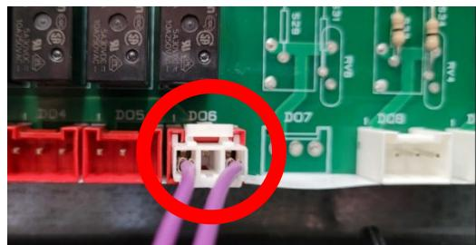
D06 has 3 outputs - 1 corresponds to neutral and 3 corresponds to phase. It is 220 V AC output.
