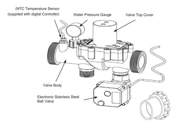
The Pool Interface Valve has an electronic stainless steel ball
