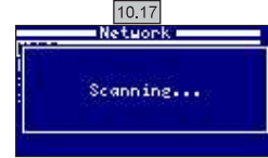
10.17 Select the desired network that the WIFI module can access. Enter the password in the pop-up keyboard. Scroll up and down with the up/down keys and left to right with the plus/minus keys. To select a letter press OK.
