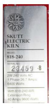
Skutt 818-240 Number of Sides - 8 Kiln Depth - 18" Kiln Voltage - 240 Volts Kiln Phase - Single
