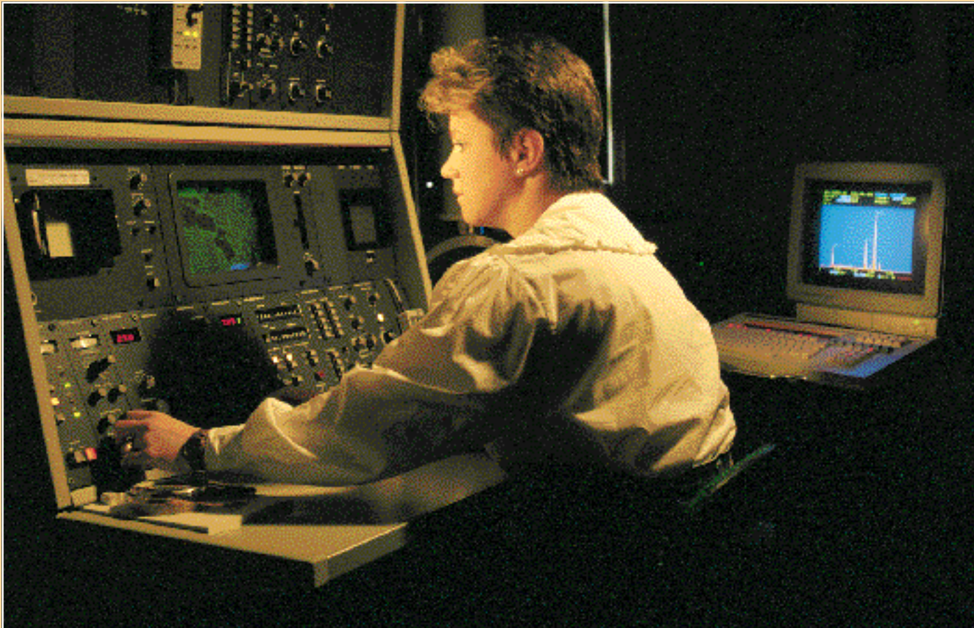
Fig. 29 The Scanning Electron Microscope is a powerful tool for material development and trouble shooting.
