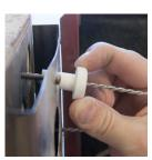
19. Put a porcelain insulator back on the element pigtail. You can reuse the old ones if they are in good shape or use the new ones included with the
