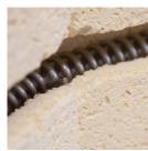
18. A pin placed correctly in the element channel.
