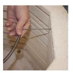
14. Push the pigtail at one end of the element through the terminal brick and into the control box. It does not matter which end you start with.
