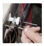
25. After you make sure the pigtail is pulled out and the insulator is pushed in cut the element pigtail so only 5/16" sticks out past the insulator.
