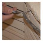
8. Remove the old element. Start and one end and pull the pigtail out from inside the kiln. Go slowly and look for missed pins.
