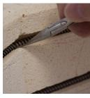
17. Keep pinning, you're not done yet! This picture shows an element pin when it is almost seated completely. Notice the angle.
