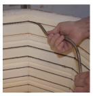
15. Install the element in the grooves. Skutt elements are pre-bent and you will notice they curve to fit the angles of the brick. Insert the other pigtail after installing the element in the groove.
