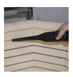
10. Vacuum the element channels. If you see any chunks of glaze or bisque stuck to the channels scrape them out and vacuum out the pieces.
