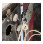
4. Cut the feeder wire just in front of the barrel connector. Save as much wire as possible. Replacement wires are available if needed.
