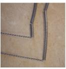
13. Start installing the new element. The two ends of the element are slightly different. Match the bends in the elements with the bends in the brick.
