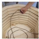
9. Remove the rest of the element from the kiln being careful not to damage the firebrick.
