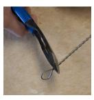
12. Cut the loop off both ends of the new element. The loop is leftover from the manufacturing process and you will not need it.
