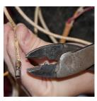
23. Crimp the connector onto the wire. Make sure the dimple is on the BOTTOM of the connector. The bottom is the closed side with no seam.
