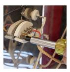
10. Replace the two screws that hold the thermocouple block to the kiln. You didn't lose them, did you?
