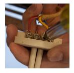
8. Tighten the two screws that hold the thermocouple into the block. Be careful not to overtighten. It's possible to crack the porcelain block
