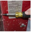
2. Remove the screws from the left side of the box. Skutt kilns have a hinged box which is held closed by 3-6 phillips screws depending on the model.
