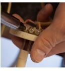
5. Loosen the two center screws on the block that are holding the thermocouple. You do NOT need to take the screws all the way out.
