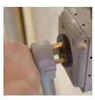
12. Plug the kiln back in and fire away! Monitor the kiln for the first few minutes to ensure the temperature is rising and if not, your thermocouple is installed in reverse.
