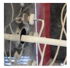
9. Slide the new thermocouple back into the kiln. The block should be pushed right up to the metal heat shield.
