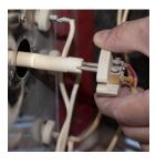
4. Slide the thermocouple out of the kiln. The porcelain block is still attached at this point.
