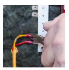
4. Use a pair of needle nose pliers to pull the thermcouple wires off the terminal strip. Do NOT pull by the wires.
