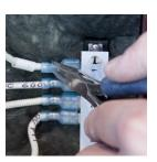
3. Use a pair of needle nose pliers to pull the blue tabs off the terminal strips. Do NOT pull by the wires.
