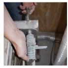
10. Pull the lid pivot bar out while supporting the springs. Note the way the torsion springs are oriented before removing them so you can replace them.
