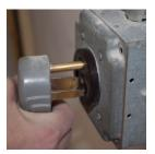
1. Unplug the kiln! If your kiln is hard wired (can't be unplugged) turn off the breaker or the disconnect.
