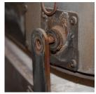
7. Lift the lid slightly and pull the lid brace off the anchor pad. Remove it from the kiln and set it aside.
