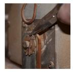
6. Start the process of removing the lid. Pull the cotter pin out of the lid brace pad.
