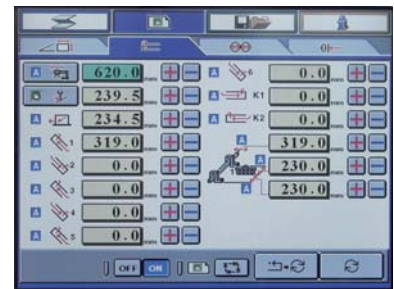
The guide and buckle positions can be fine-tuned by 0.1 mm using the + or – button.
