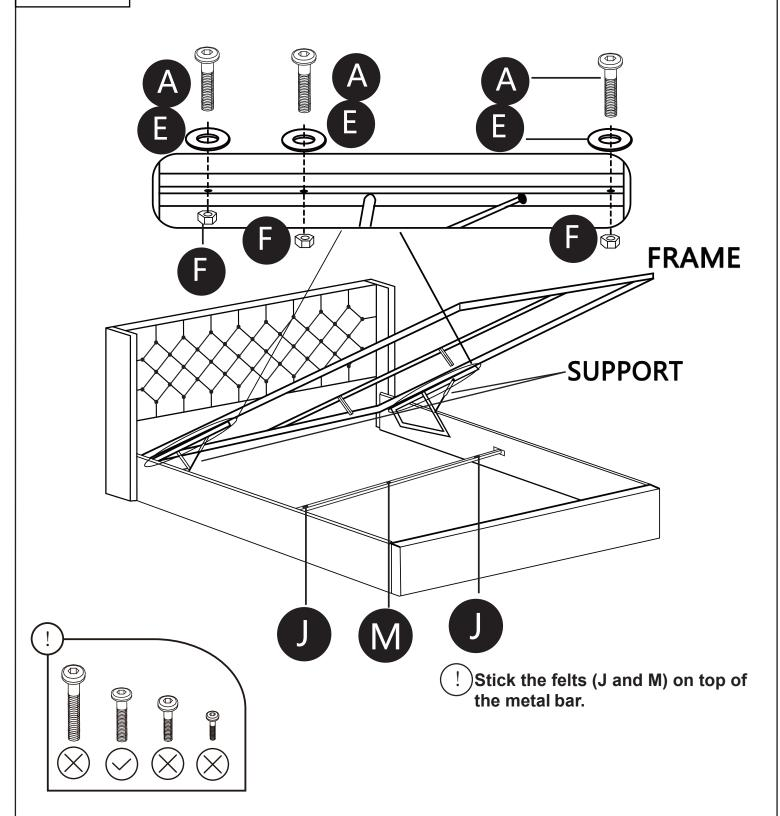
Step 12: Attach the frame that you built in the previous steps to the gas lift mechanism at a 45° angle (meaning it should be slanted as shown in the picture) using hardware A, E and F.
