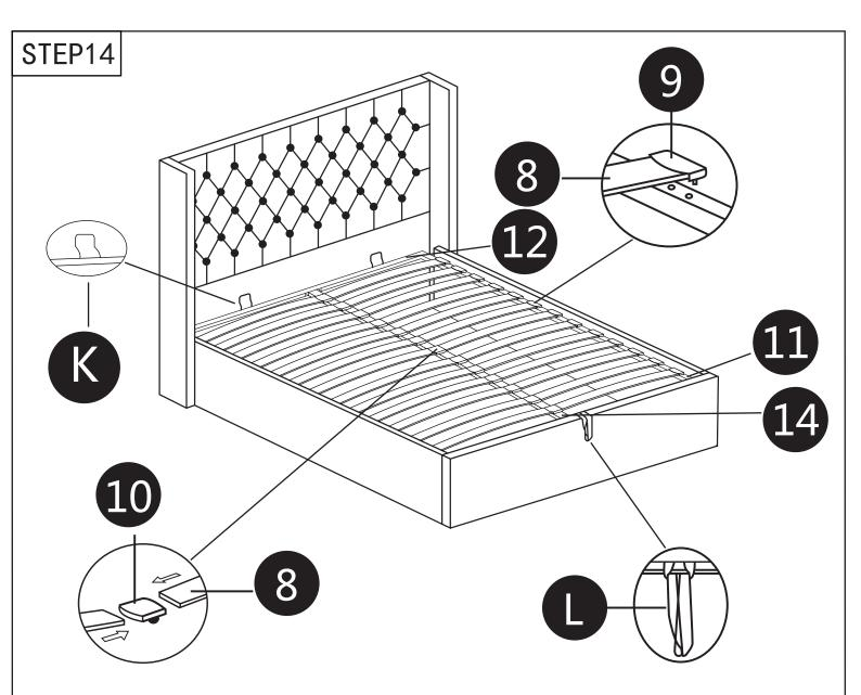
Step 14(a): Attach the slats (8) to the plastic clips and insert them into the holes of the metal bars (11 and 14). Clips open from both sides (10) will be attached to the middle bar (14), and clips open from one side (9) will be attached to the side bars (11).
