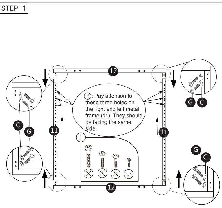
Step 1 : Attach parts 11 and 12 using hardware C and G.
