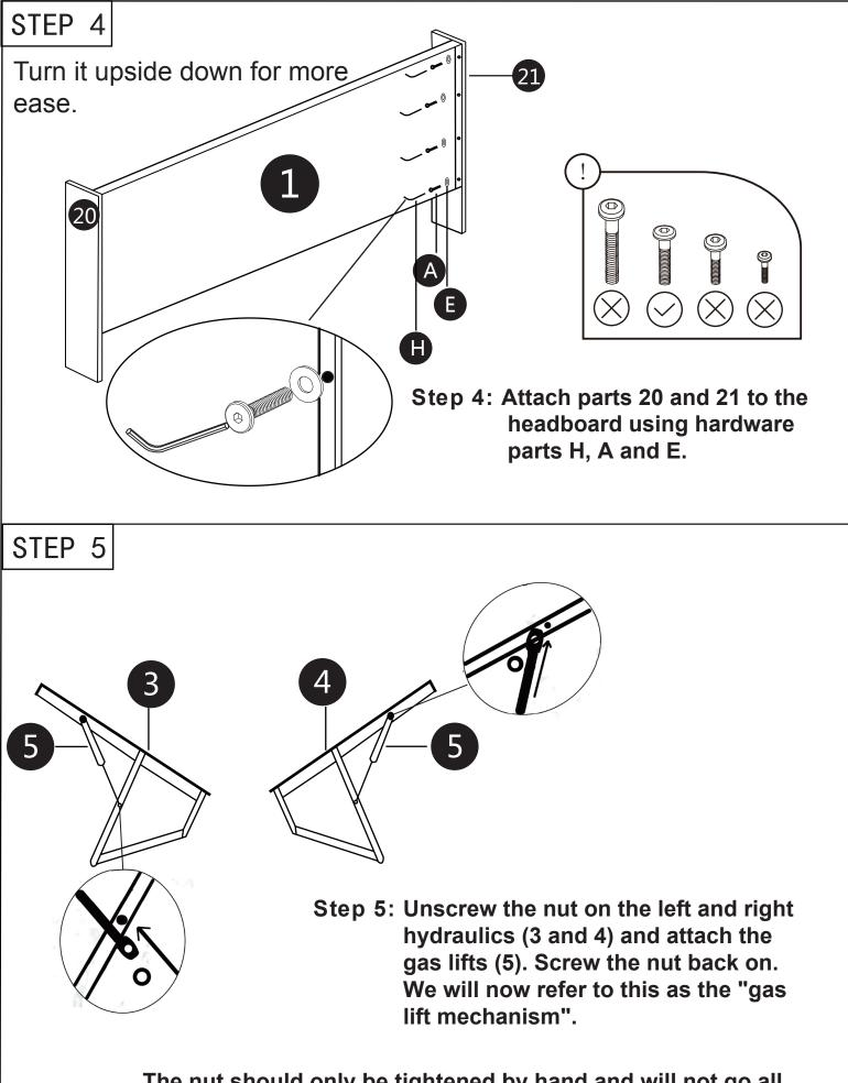
The nut should only be tightened by hand and will not go all the way in. No tools needed.
