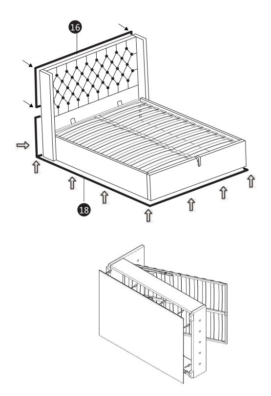
Step 15a : Attach the non-woven fabric (18) to the bed. Start from the bottom of the bed and go halfway behind the headboard.
