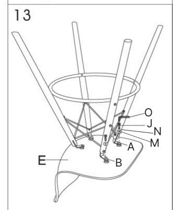
Connect the seat to the legs using "M", "N" and "J". Legs "AD" and "BD" are the front legs of the stool.
