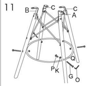
Connect Circle "Q" with the bottom holes of all the 4 legs using screw "G".
