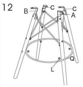
Cover all screw ends with part "L" after tightening.
