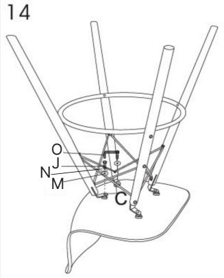
Connect the seat to the legs using "M", "N" and "J". The two "CD" legs are the back legs of the stool.
