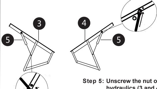
Step 5: Unscrew the nut on the left and right hydraulics (3 and 4) and attach the gas lifts (5). Screw the nut back on. We will now refer to this as the "gas lift mechanism".
