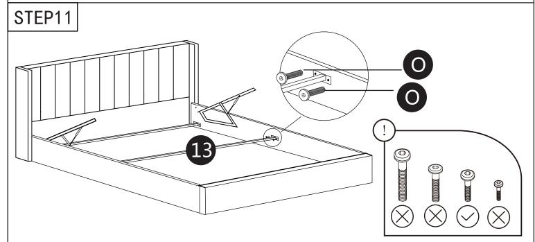
Step 11: Attach the second side rail connector (13) to the centre of both side rails (6 and 7) using hardware O.
