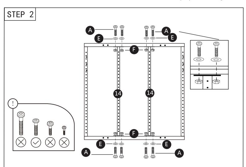
Step 2: Attach part 14 to both sides of part 12, using hardware A, E and F.
