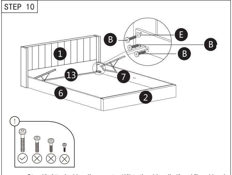
Step 10: Attach side rail connector (13) to the side rails (6 and 7) and head-board (1) using parts B and E.
