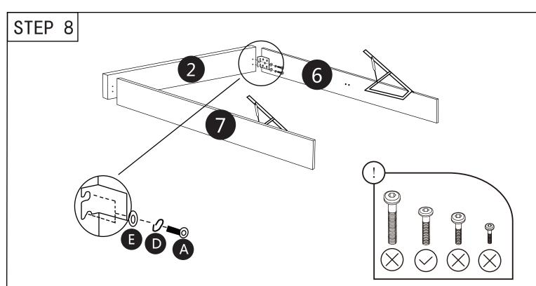
Step 8: Attach the side rails (6 and 7) to the footboard (2), using hardware E, D and A.
