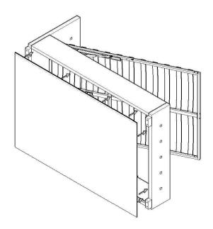
Step 15a: Attach the non-woven fabric (18) to the bed. Start from the bottom of the bed and go halfway behind the headboard.
