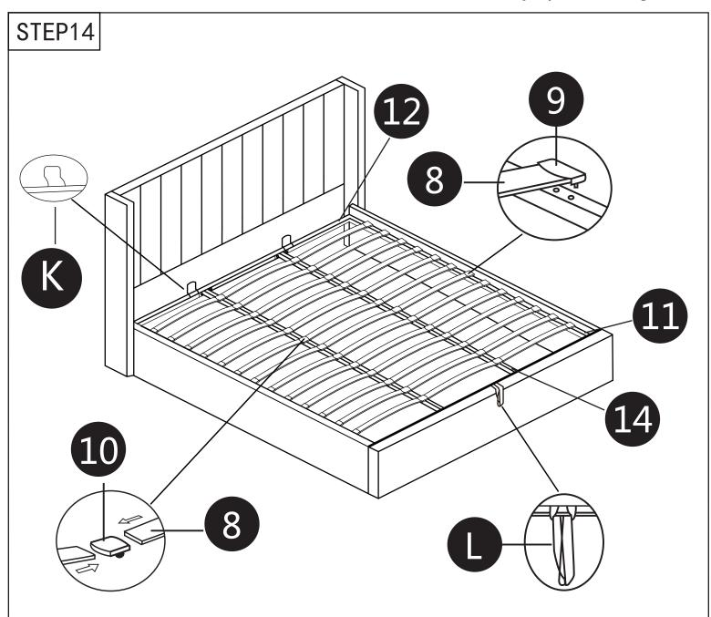
Step 14(a): Attach the slats (8) to the plastic clips and insert them into the holes of the metal bars (11 and 14). Clips open from both sides (10) will be attached to the middle bar (14), and clips open from one side (9) will be attached to the side bars (11).
