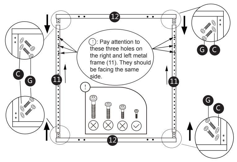
Step 1: Attach parts 11 and 12 using hardware C and G.
