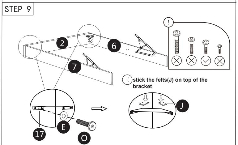
Step 9: Attach the corner bracket (17) to connect the side rails (6 and 7) to the footboard (2), using hardware E and O.
