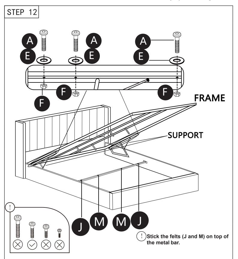
Step 12: Attach the frame that you built in the previous steps to the gas lift mechanism at a 45° angle (meaning it should be slanted as shown in the picture) using hardware A, E and F.
