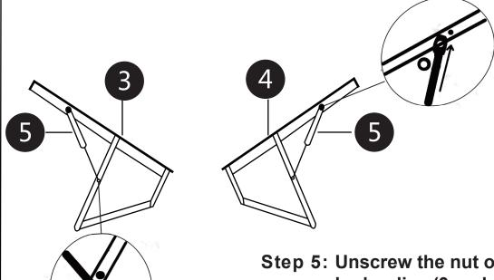
Step 5: Unscrew the nut on the left and right hydraulics (3 and 4) and attach the gas lifts (5). We will now refer to this as the "gas lift mechanism".
