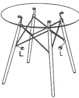
Tighten all the screws at the end using the Allen key (part K) to adjust the legs. Attach the screw caps (Part L) to all the screws.
