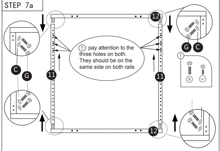
Step 7a: Attach parts 11 and 12 using hardware C and G.
