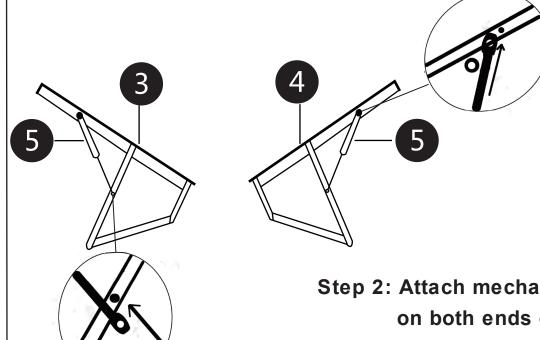
Step 2: Attach mechanism (5) to gas lift (4) on both ends on the right and left gas lift. We will now refer to this as the "gas lift mechanism".
