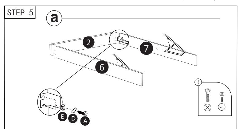
Step 5a: Attach the side rail (6 and 7) with the footboard (1), using hardware E, D and A.
