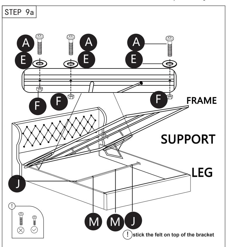
Step 9a: Attach the frame that built in the previous step to the gas lift mechanism at a 45° angle (meaning it will be slanted as the picture), using hardware C, F and E.
