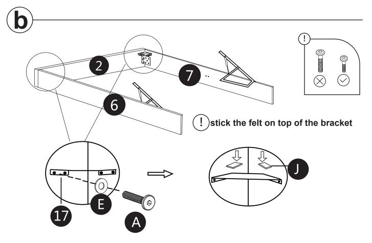
Step 5b: Attach the corner bracket (17) to side rail (6 and 7) and footboard (2), using hardware E and A.
