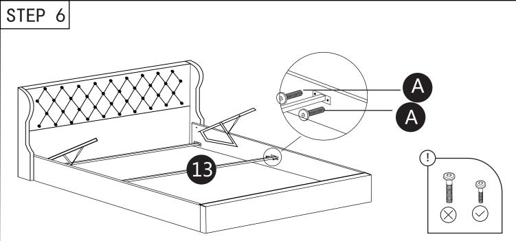
Step 6: Attach the center support to both the side rails, using hardware A.
