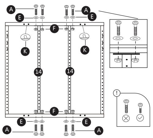
Step 7b: Attach part 14 to both sides of part 12, using hardware A, E and F.
