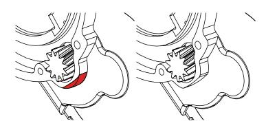
3. Using a file, carefully remove material to the scibbed in line making it the same shape as the Lekkie Drive Cover HD. You may also need to trim the paper gasket.
