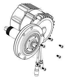
1. Using a 4mm hex unscrew the 6 screws holding on the stock cover and remove.
