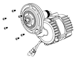
4. Install paper gasket then slide the new drive assembly in. Clean, apply Loctite 243, and install the 6 M4 drive cover bolts. Tighten to 6Nm.
