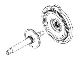
**3. Slide the remaining axle assembly in.** Note: Grease all touching surfaces to make maintanance easy.
