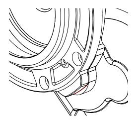
1. Place the Lekkie Drive Cover HD on the motor and trace pinion cover edge.
