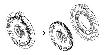
4. Screw 3 M4 screws into the back side of the drive gear until they are touching the bearing. Start turning one screw one turn, then the next screw once, then turn the next screw one turn, then the next. Repeat untill the gear is removed.
