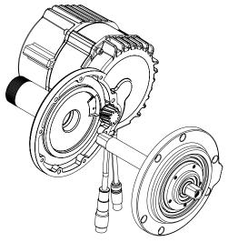
2. Tap the axle from left side of motor, loosening the drive assmebly and remove assembly.
