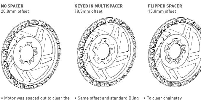
• Motor was spaced out to clear the frame
