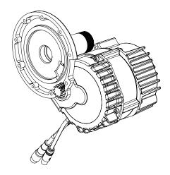
2. Remove the Lekkie Drive Cover HD. Note the scribbed in mark showing what you will be removing.
