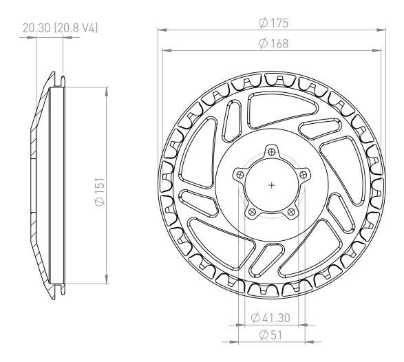
Note the package includes a 2mm Spacer so that you can space the Bling Ring out to the same offset as the original Bling Ring offset. We decided to offset the Bling Ring an extra 2mm so that useres could try get that perfect chainline for the 73mm BB frames. If you are building a 73mm BB frame try installing without the spacer. You should have at least 1.5mm gap between the ring and chain-stay.
