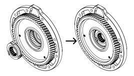
**1. Press the main drive gear into the new bearing in the Lekkie Drive Cover HD.** Note: Grease the inner edge of the bearing.
