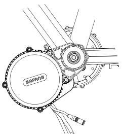
5. Rotate the motor up until it stops on the frame., hold and tighten the Screw On Cup with the 16 notch socket to 25-30Nm. Then tighten the plate bolts to 9Nm.
