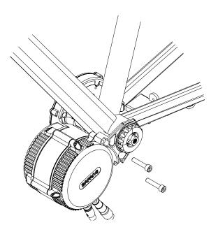
**4. Loosely screw in the 2x M6 Plate Bolt.** Note: If you are installing on a 92mm wide frame use a the Motorspacer. If you are installing on a 48mm oter diamter motor you will need to add a 2mm spacer.
