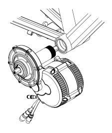
2. Grease motor body shaft and slide through from the right hand side.
