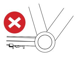
Carbon frames oftern have alot of reinforcing under the BB of the frame the motor can not fit
