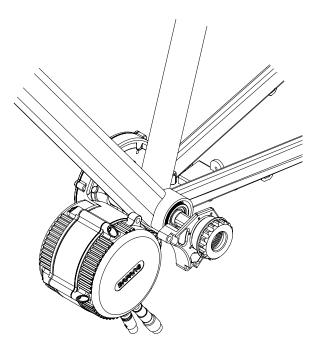
3. Grease the inside of the frame on the left side. Slide the Motor Plate onto the Screw On Cup and screw onto the motor loosely so that the motor can still rotate.
