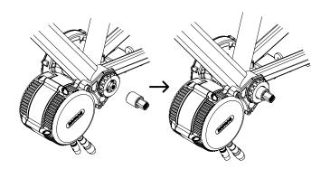
6. Grease the left side axle and slide on the Axle Extender.
