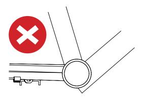
Protruding tubes, chain guide mounts or welds may get in the way of the motor.
