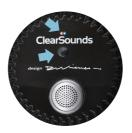
**STEP 3:** On the Mic, press and hold BUTTON until light flashes red and blue.
