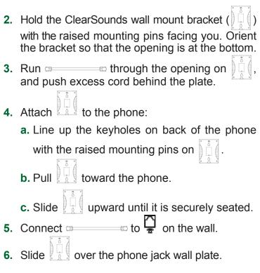
To simply hang the phone on the wall This method requires two self-tapping screws (not included).
