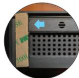
**STEP 2:** On the underside of the lifter, remove the paper backing from the two pieces of tape.
