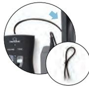
**STEP 2:** Connect the short Hub-to-base cable to the phone base port where the curly cord had been connected.
