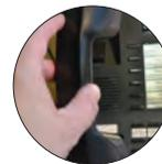
**STEP 4:** Confirm that you hear a dial tone in the handset by manually lifting the handset from the base.
