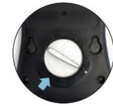
**STEP 6:** **If you do not hear a noticeable dial tone:** On back of QH2, click the dial until you hear a dial tone. On the hub, slide the VOLUME slider or TONE slider until you hear a change in volume and tone quality. Repeat these steps until you find a compatible setting.
