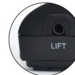
**STEP 4:** Connect the L-shaped connector to the LIFT port on the bottom of hub...
