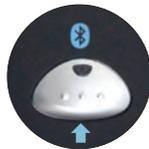
**STEP 2:** On the hub, press and hold the multi-function button (MFB) until the blue and red lights flash.
