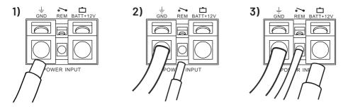
Remember that if you're using the high level input connection on the MAX A2-100.2 model, you don't need to connect the REM (remote) cable to the amplifier.
