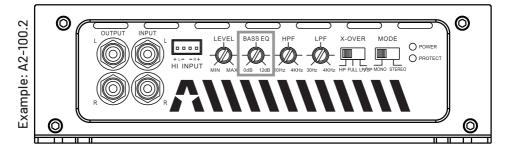
If everything is tuned correctly and the level/gain has been set, the BASS EQ should remain in default (0dB). This function will apply level/gain at 45Hz centre frequency. Be adviced that equing the bass from 0-12 dB is a lot, an increase of +3dB doubles the output! If used incorrectly, this can permanently damage your subwoofer.
