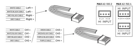
Use the right speaker cable for the job! Make sure to use the recommended size, and follow the polarity of the speaker wire from the speaker to the amplifier.
