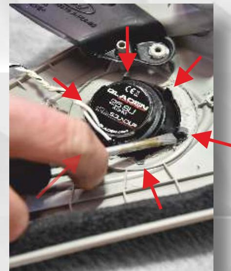
*To attach the tweeter insert, bend all the metal tabs on the back with a screwdriver and press them tight.
