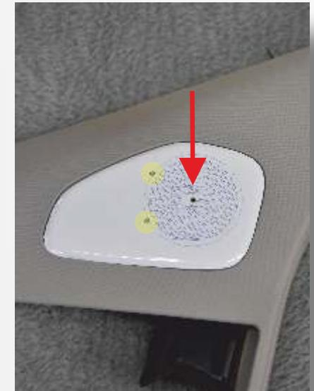
*Position the enclosed sticker template in the center of the original grille. The hole in the middle should match the central hole in the original grille. The two holes on the edge of the template will be needed later for adjustment.*
