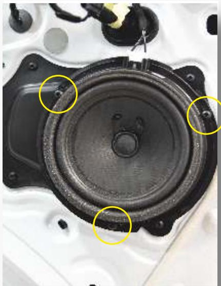
*To remove the original loudspeaker, please disconnect the connector plug. The marked screws must then be loosened and removed. Remove the speaker from the holder.*
