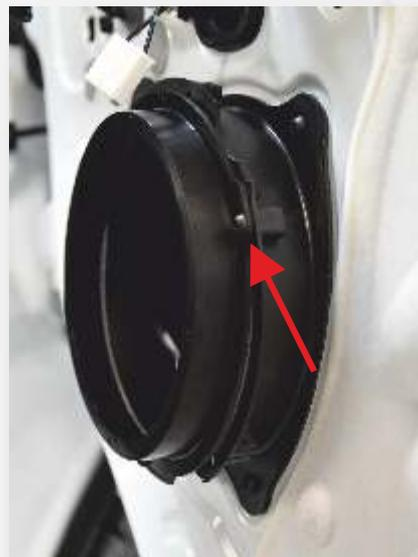
*Fit the new loudspeaker adapter ring onto the loudspeaker opening in the door. Use the vehicle manufacturer's previously loosened screws for this.*
