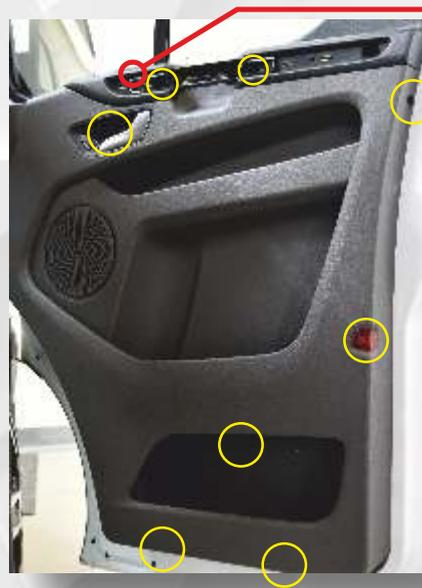
*The yellow marked fields contain fastening screws that need to be loosened.*
