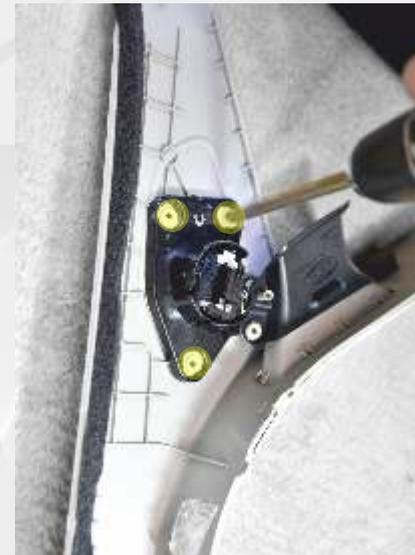
*Remove the original tweeter bracket. To do this, carefully drill out the plastic welds with a 10 mm drill bit.*
