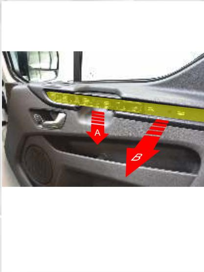
*To remove the door trim, use a plastic tool to click out the upper handle trim (B). To do this, a plastic latch in the lower part of the handle must first be pulled downwards (A). There are two fastening screws under the main trim panel.*
