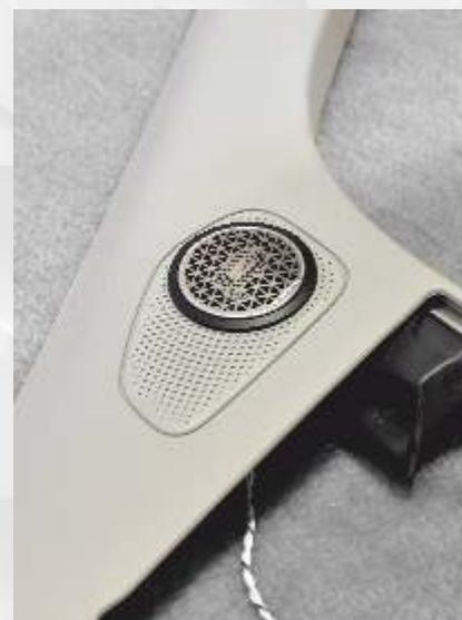
*Insert the tweeter into the opening and check that it is flush with the edge.
