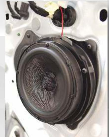
*You can now screw the speaker in place and reassemble the door.*
