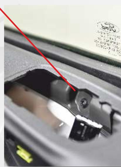
*Caution: There is another fastening screw in the door trim behind the power window switch. To do this, carefully lever out the switch using a plastic tool.*
