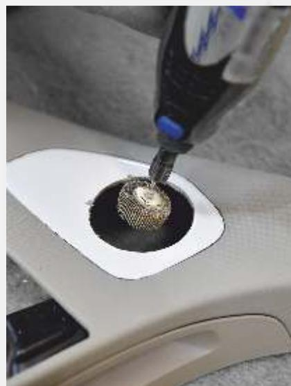
*Carefully cut out the opening for the tweeter using a motor sander.
