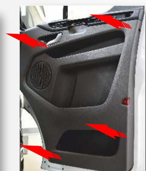
*Pull off the door trim using a plastic tool. Disconnect all cable connections and the door opener cable before finally removing the door trim.*
