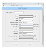
In the SRT interface of the encoder, select Listener for the mode, and fill in 4201 for the Source Port (the same as the decoder's Destination Port).
