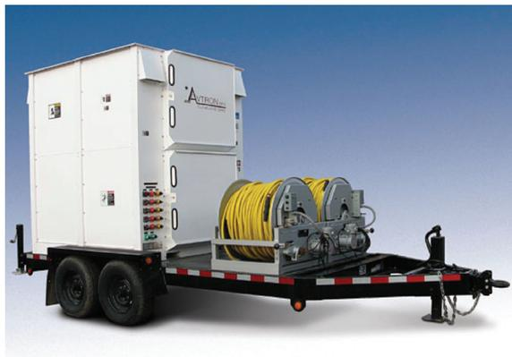
**Automatic auxiliary loading:** This solution is usually used only when the diesel generator set is the primary source of power. The “auxiliary load bank” will be switched into the system when only the lighter loads are present and switched out when the larger load is connected.
