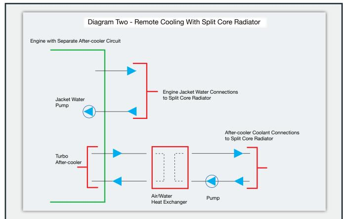
Ventilation - The generator installation, especially an inside location, requires adequate ventilation in order to provide sufficient air for cooling, combustion, and removal of radiated heat from the generator set. When there are limitations to the amount of air that can be discharged into and from the generator location, remotely mounting the radiator allows a 50% drop in the quantity of air required in the generator room. (Continued over)
