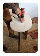
Attach the 2 wide slats (seats) and the remaining rods with the screws.
