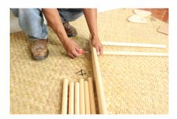
Verify that all rods on both sides are aligned. If you have a lightly twisted rod unscrew it, rotate it and screw again until it is fully aligned.
