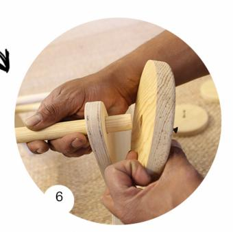
Apply a drop of glue on each end of this rod for it will provide the wheels a perfect hold.
