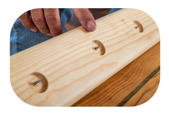
Start placing the rods in their corresponding spots, spinning them to ensure the screw tips are gripping the wood. Make sure they go all the way into the slots.
