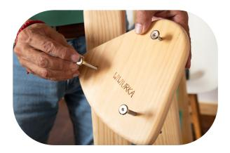
Then screw in the assembly screws using the allen key, this will fasten the pieces at the top together.
