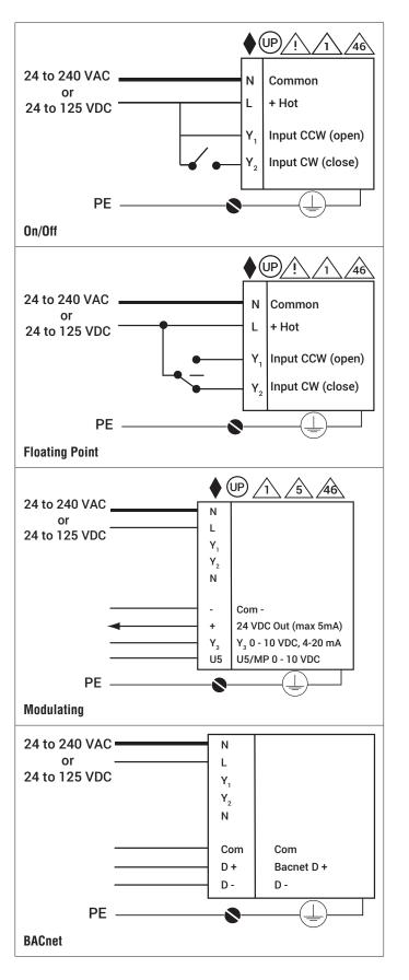
Modulating, Electronic Fail-Safe, 24...240 V, NEMA 4X with BACnet
