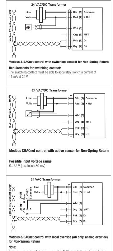
If no sensor is integrated, then connection 3 (Y) is available for the protective circuit of a local override control. Options: CLOSED, Vmax, OPEN
