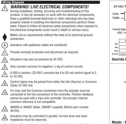
A Master-Slave wiring required for piggy-back applications. Feedback from Master to control input(s) of Slave(s).
