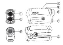
The HX-1200T range finder emits invisible, eye safe, infrared energy pulses. Sophisticated digital technology instantaneously calculates distances by measuring the time, which it takes for each pulse to travel from the rangefinder to the target and back to rangefinder.
