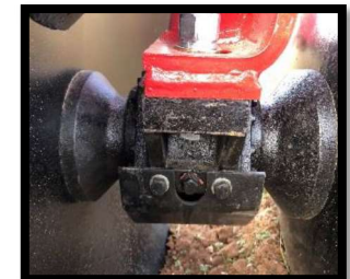
OIL BATH BEARING WITH DUO-CONE SEALS FOR EASY MAINTENANCE
