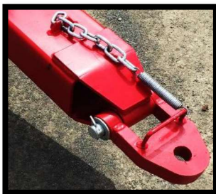
SIMPLE CHAIN AND SPRING ASSEMBLY ON HITCH ALLOWING FOR EASY HOOKUP
