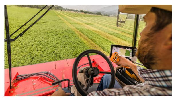
**MF Guide** is Massey Ferguson's complete guidance system for hands-free steering, now available factory fit on WR windrowers. MF Guide helps you eliminate skips and overlaps while letting you focus on the quality of your windrow instead of driving. A choice of two different receiver systems is available — NovAtel and Trimble — while a selection of signal-correction services offers the exact level of accuracy you need.
