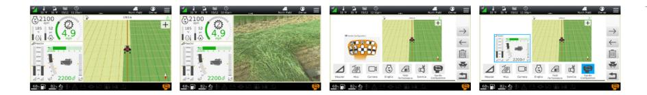
**ELECTRONIC HEADER SPEED CONTROL** Smart machine management adjusts hydraulic flow to the header when cutting high-yielding areas or navigating steep terrain, ensuring consistent header rpm for even cutting and conditioning.
