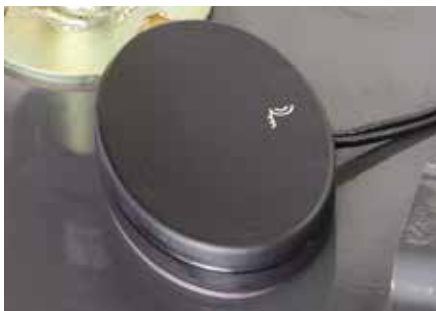
AGCOMMAND combined GPS & GSM antenna.
