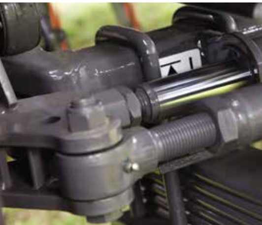
Rear axle hydraulic steering lock.
