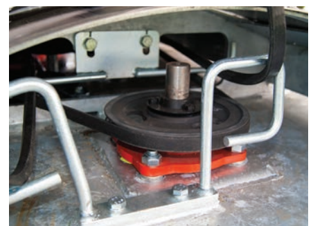
Improved belt engagement on larger drive pulleys to reduce slipping in heavier grass conditions.
