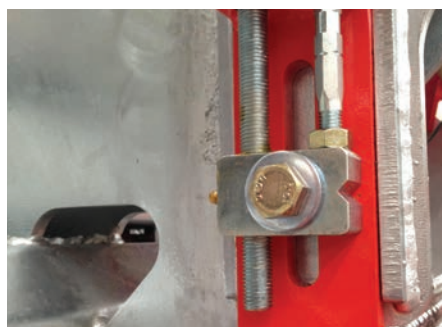
Adjustable rollers provides precision height control. Cutting height indicators for even height settings.
