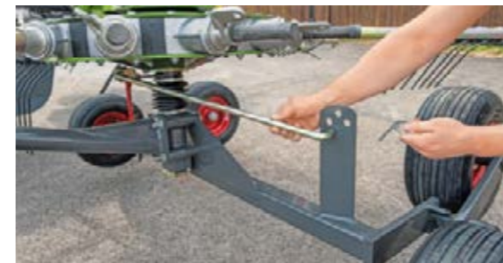
Whether the forage is long and heavy, or short and light: The cam track can be easily adjusted to suit the harvesting conditions.
