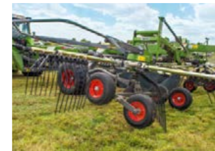
When lowering on headlands, the back wheels touch the ground first, followed by the front wheels. When lifting, the rotors are raised first at the front. This Jet-Effect protects the sward.
