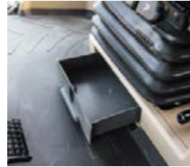
■ There is a storage compartment under the driver seat. That ensures there is order in the cab.
