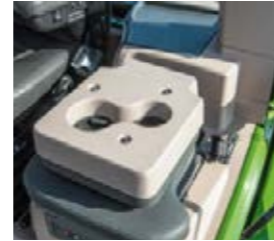
■ The instructor seat with seat belt serves as a bottle holder when folded down.
