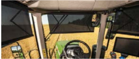
■ The roller shades on all sides protect the operator from glare and neatly disappear into the roof liner.
