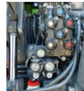
The hydraulic connections are marked in colour. This way, you can couple devices quickly and safely.
