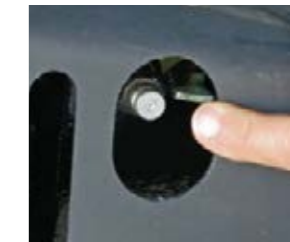
□ The pressure for pre-tensioning the rolling track can be comfortably adjusted from the side by means of a connection.
