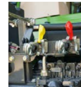
The dual-circuit air brakes also act on the trailer when the parking brake is applied.
