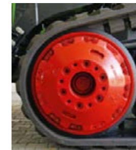
The front idlers can be ballasted with up to 1,580 kg.
