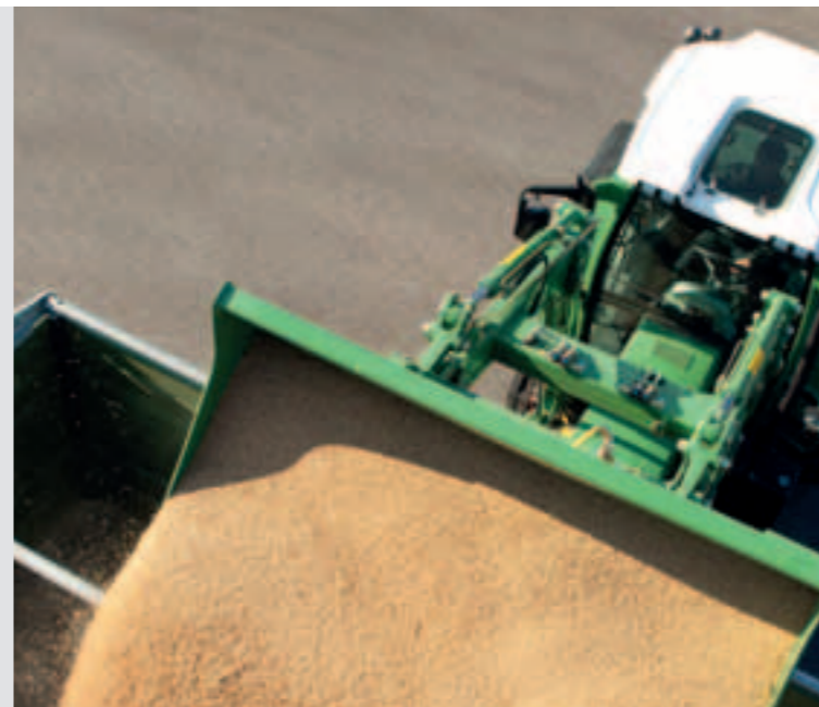
The roof window, which is standard on the 200 Vario and optional for the 300 Vario, provides an optimum view to the raised front loader.
