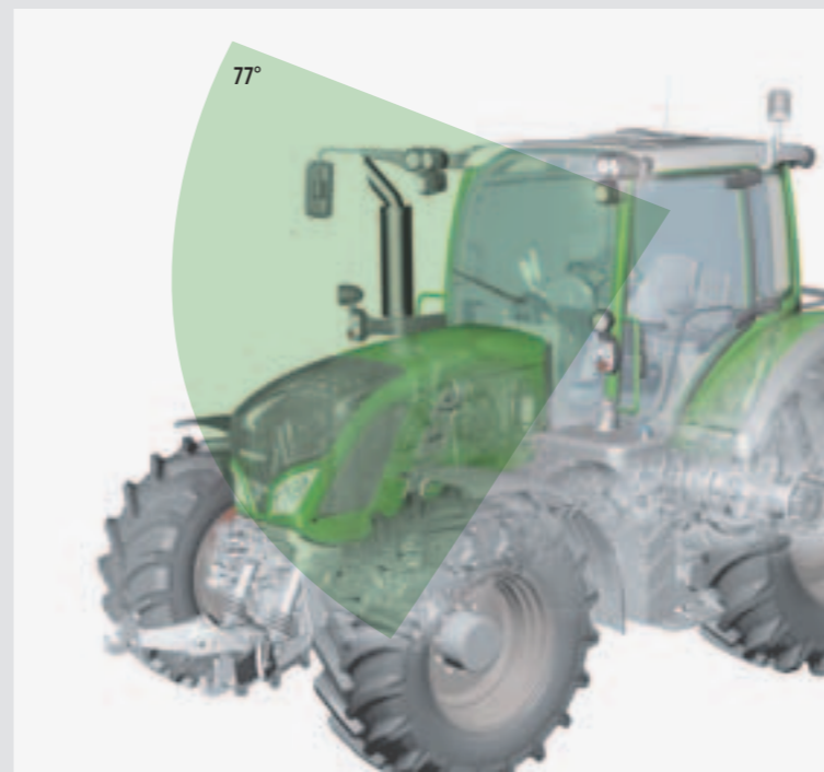
The new 700 Vario is fitted with the VisioPlus cab, which features a front windscreen that curves up into the roof. It triples the upward viewing angle and provides a full view of the front loader, even when it is fully raised. The downward sight lines have also been optimised and provide an excellent view to the wheel arches.
