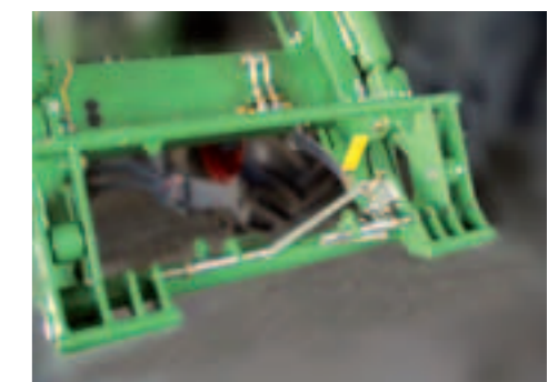
The standard-equipped semi-automatic attachment lock is operated with a single lever.
