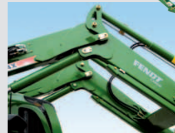
Mechanical self-levelling – compact design through Z-bar linkage
