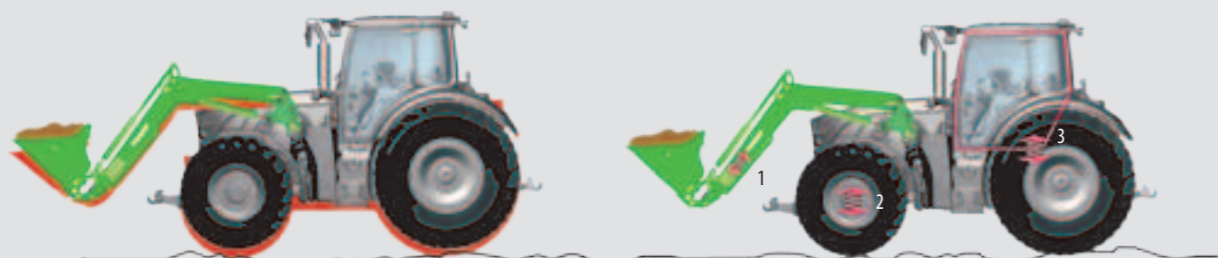
Front loader without damping system: shock loads are transmitted to the tractor.
