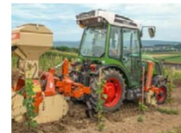
Inter-axle mounting for efficient use of flexible implement combinations.
