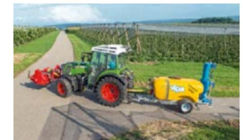
Efficient combination of processes. With the 540E/750 front PTO, you can drive the mulcher at the operating speed, though the sprayer in the rear and the tractor operate at a reduced engine speed.
