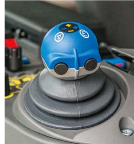
■ The third and fourth control circuits are conveniently activated via a button or switch on the electric crossgate lever.
