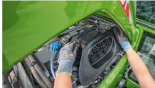
The easily accessible air filter with pre-cleaner delivers maximum performance in air flow and filter life. It is compact and particularly well-sealed. Benefit: low maintenance.
