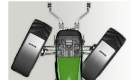
The VarioActive function allows you to achieve full steering lock with just one turn.
