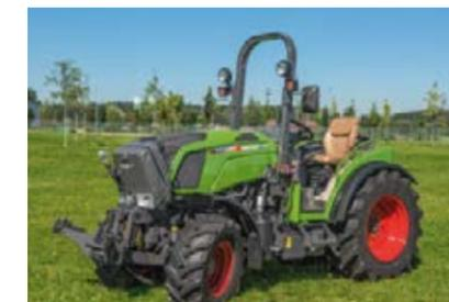
For use in glasshouses or in restricted spaces, Fendt offers variants without a roof and with a roll bar.
