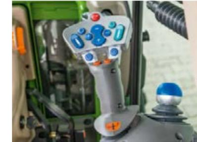
Four double-acting valves on the right-hand and two valves on the left-hand side, together with return flow and cross connection, permit optimal supply of high-level hydraulic combinations. You can use up to 3 mounts at the same time for time and cost-saving combinations.
