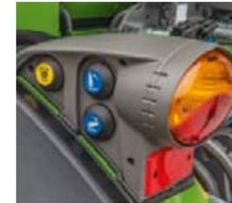
■ The external controls for hydraulics and PTO are located on the rear mudguards.
