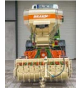
The lower links can be adjusted to the left and right using the two hydraulic cylinders, and guide the rear implement precisely along the row. Free floating is possible in the floating position.
