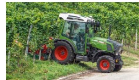
The PTOs operate independent of the road speed. This lets you drive slowly when mulching a dense uncut crop, and drive faster, continuously, without changing gears or switching off, in sparse crops.
