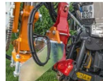
The mounting plates integrated in the front linkage always provide a stable and secure base for heavy front-mounted implements.
