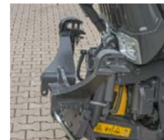
The lower links of the fully integrated front hydraulics can be folded compactly in just a few steps. The compact design makes the 200 Vario particularly manoeuvrable even with a front attachment.
