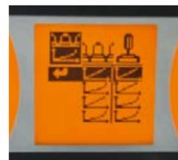
■ The sensitivity of the hydraulic control units can be easily adjusted in the display.
