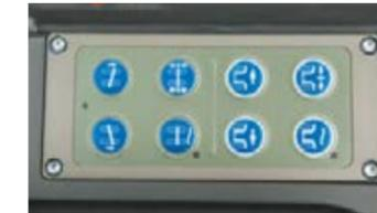
You can control the lateral and tilt adjustment of the swinging power lift, as well as swing and lock, with the push of a button. The tilt adjustment display always show you the setting to suit your application.
