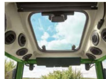
The roof window, integrated as standard, provides the best visibility for all types of overhead work. The window can be opened upwards for ventilation in the cab. A sun shade protects against intense sunlight.
