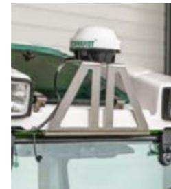
Position-based GPS steering systems provide accuracy down to 2 cm in the Fendt200V/F/P Vario.
