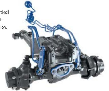
Soil protection is a combination of many factors: Swinging power lifts with a wide and deep traction point at the front, 4WD and automatic differential lock, levelling box and anti-roll control on the front axle. Optimal traction under any conditions.
