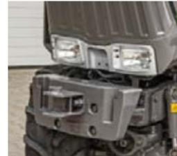
□ Without the front linkage, there is an option to fasten additional ballast directly onto the frame.
