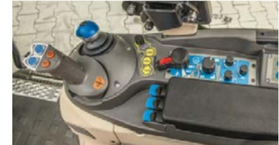
The Stop&Go function on the reverse gear stick brings the FendtV/F/PVario to a stop, and accelerates it in the direction of the rocker. Perfectly smooth and gentle on the soil.
