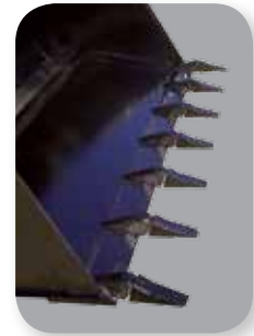
Multi-purpose bucket with ground engaging teeth fitted
