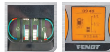
The digital AdBlue displays may state 'UREA' or 'DEF' (Diesel Exhaust Fluid)
