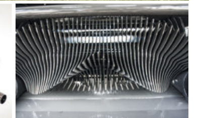
XtraCut25 Rotor - With cutting system: up to 25 knives
