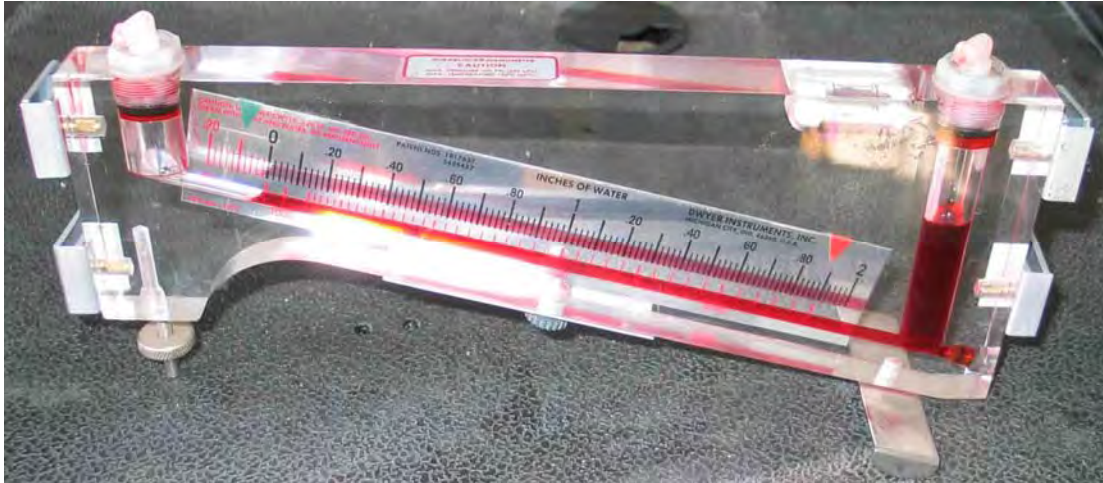
Figure 3.6. Inclined manometer used to measure the pressure difference on the LFE.
