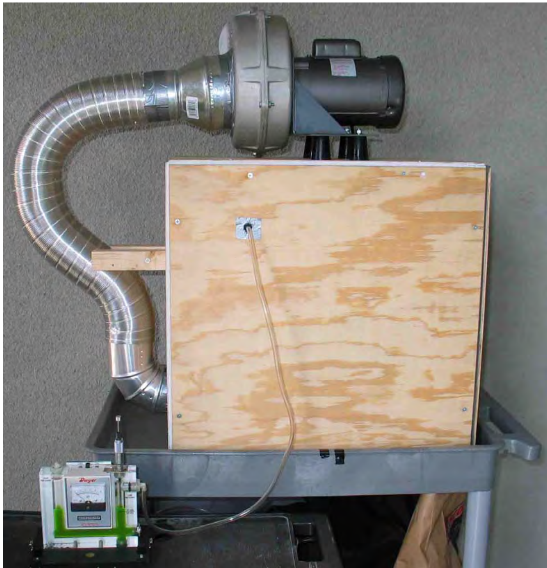
Figure 3.5. Experimental apparatus with the micromanometer used to measure the pressure difference across the door, shown here with the flexible ducting installed for the ultimate seal failure test.
