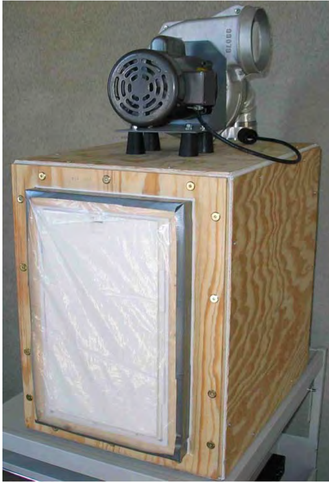
Figure 3.3. Experimental apparatus with a pet door sealed for a peripheral leakage test.
