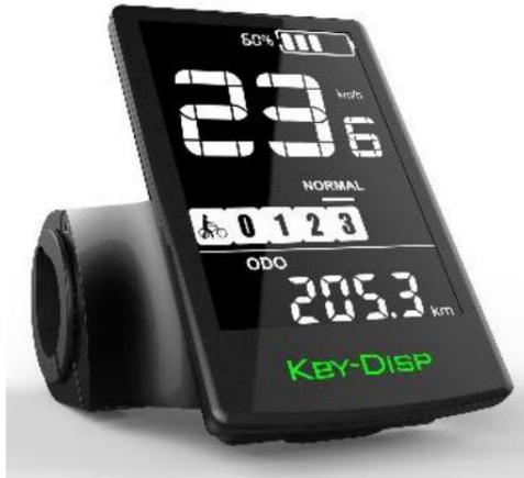
The KD716-V instrument matches the K5 buttons and has 5 buttons: ON/OFF, i-button, plus-button, headlight-button, and minus/boost-button; in subsequent descriptions, the ON/OFF button is replaced by the word "ON/OFF"; the i-button is replaced by the word "i"; the plus-button is replaced by the word "+"; and the minus/boost-button is replaced by the word "-".
