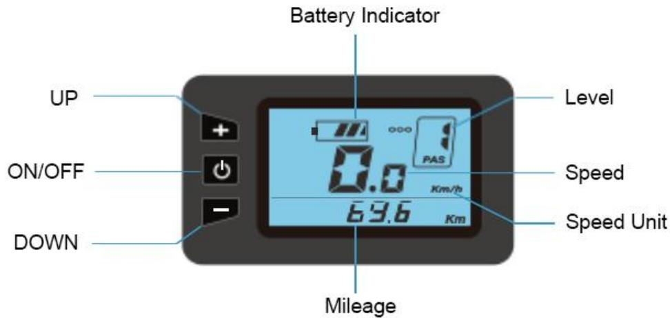
There are three buttons on the instrument, including on/off, plus/headlight, and minus/boost; in the instructions that follow, the on/off button is replaced by the word "ON/OFF", the "+" button is replaced by the word "UP", and the "-" button is replaced by the word "DOWN".
