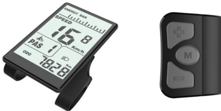
The main body of the button is made of PC material, and the key part is made of soft silicone, all black. There are three buttons on the button. These include the power-on mode button "M", the plus button "+" and the minus button "-". In the subsequent manual, the button "M" is replaced by the text [MODE]; the button "+" is replaced by the text [UP]; the button "-" is replaced by the text [DOWN].
