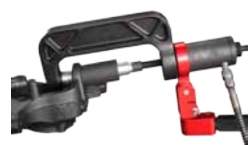
Ball joint removal using “C” Clamp
