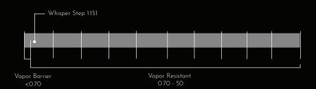
Whisper Step is semi-permeable, which means vapor can pass up through it
