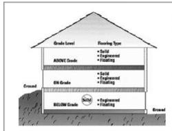
If the soil surrounding a structure is 3 inches or more above the floor of any level, consider that level below grade. This includes walk-out basements. In addition, the surrounding soil should be sloped away from the structure.
